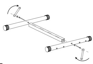
Put four round tubes into the round holes at the end of the base fixed with screws
